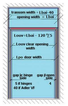
With this flush-mounted transom construction, use a glazing bead profile on the hinge side.
